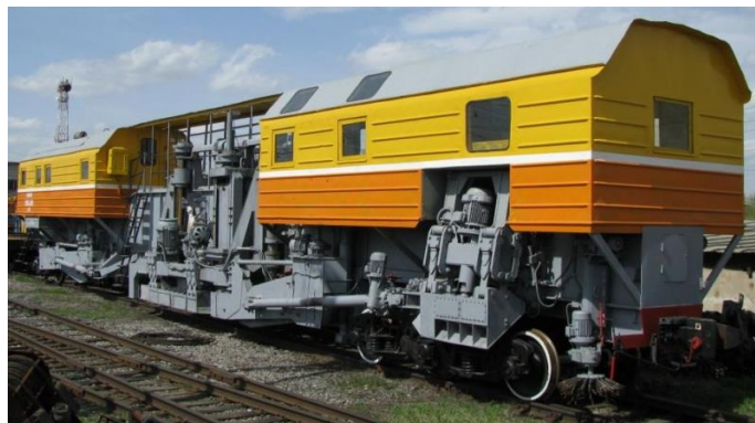
Figure 1 – Straightening and tamping and finishing machine
