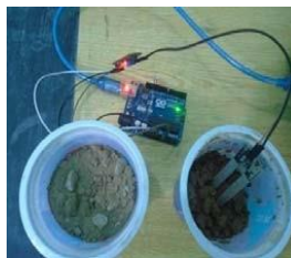
Figure 5 – IoT Moisture Content Testing
